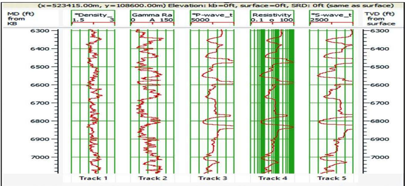
Fig. 3: Isomu\_1 showing Gamma ray log, Density log, Compressional and shear velocity logs
