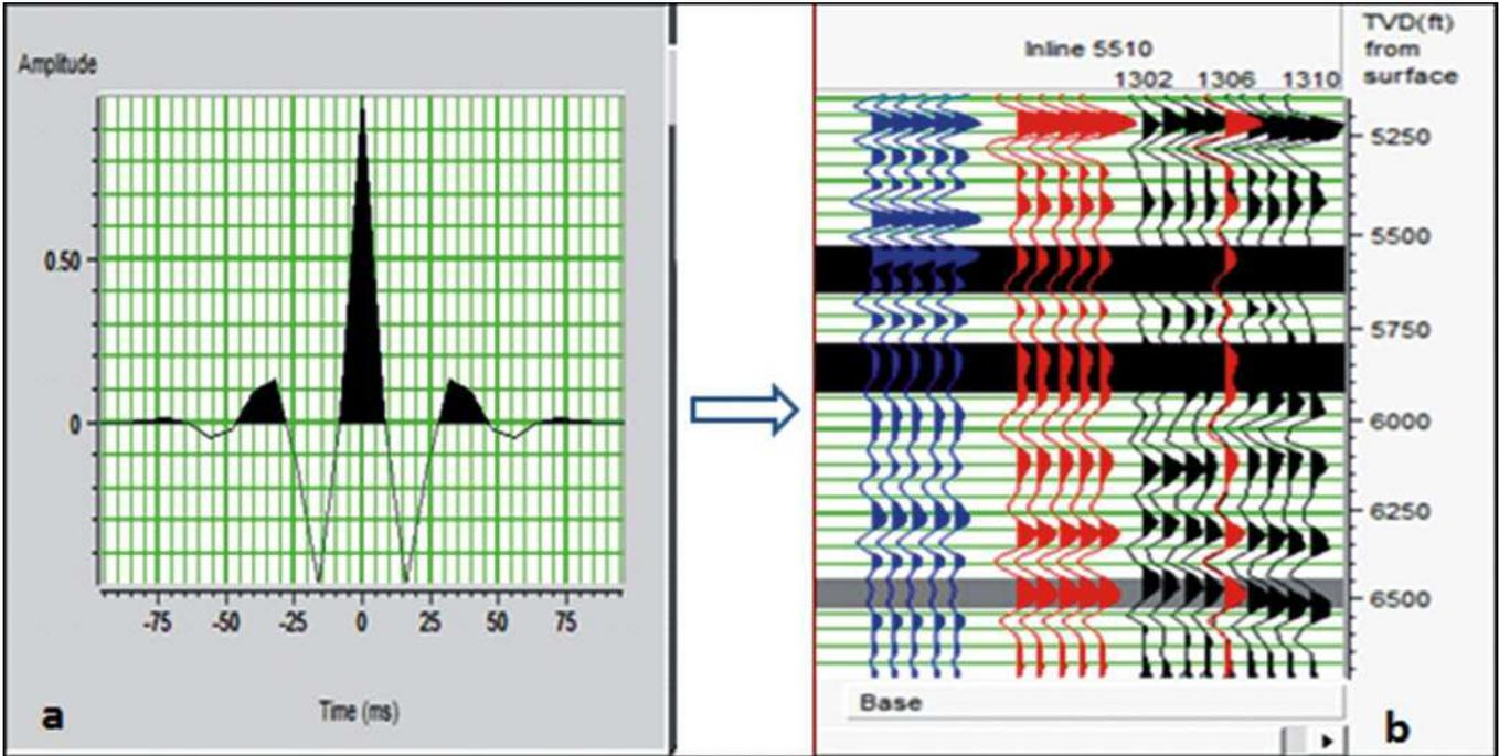
Fig. 2a-b: (a) Statistical wavelet time response and (b) seismic to well ties.
