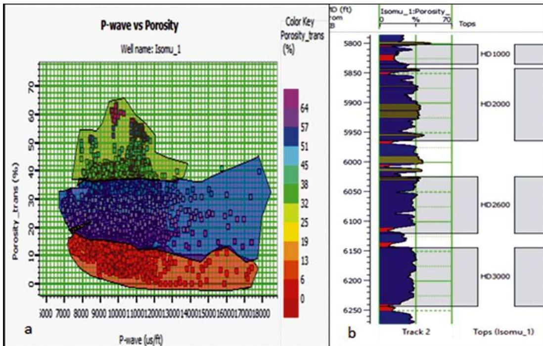
Fig. 4a-b: The cross plot of porosity versus velocity and (b) cross-section of the porosity in the Isomu\_1.
