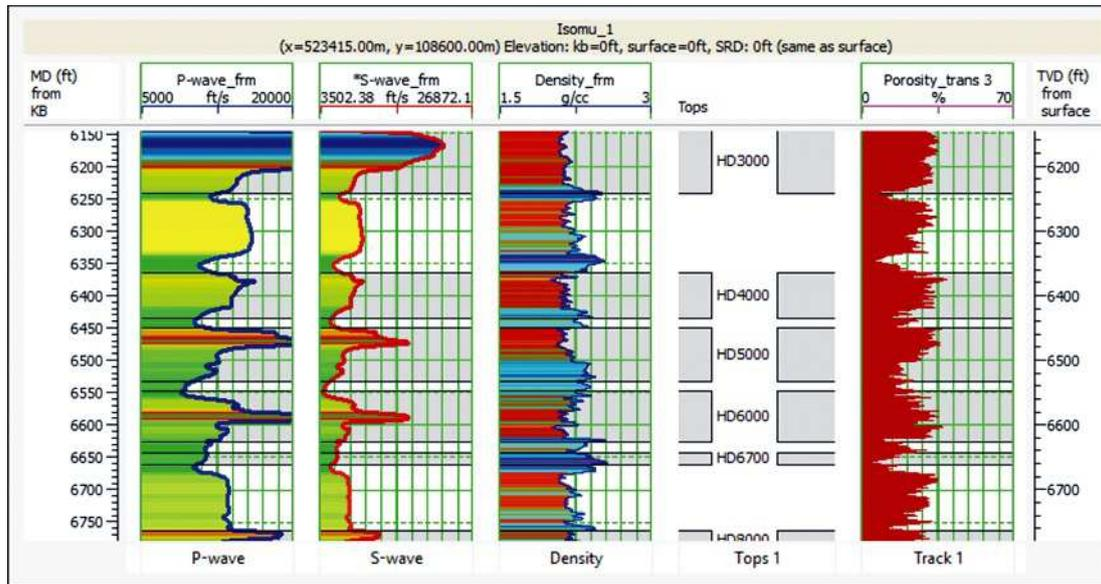
Fig. 5: The well log response to fluid replacement modelling
