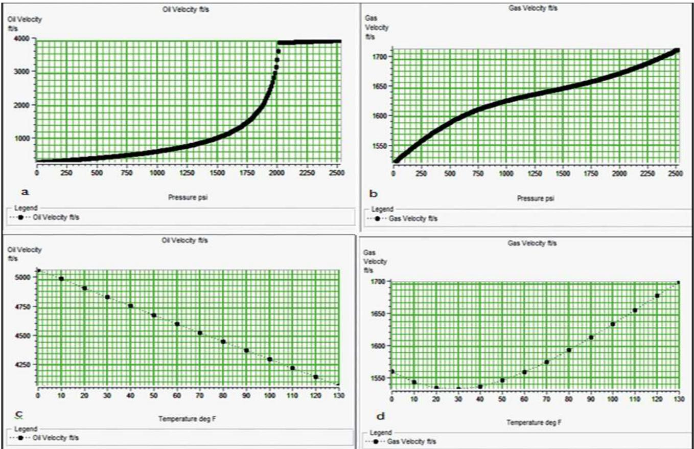
Fig. 8a-d: Effects of fluid properties on velocity under temperature and pressure
