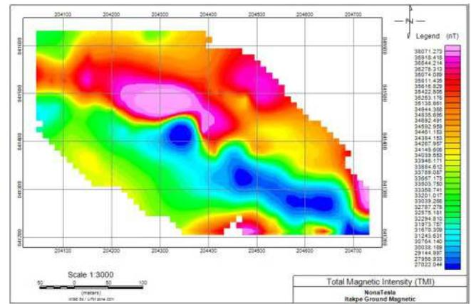
Fig. 4: Total magnetic intensity map of the Itakpe iron ore field.
