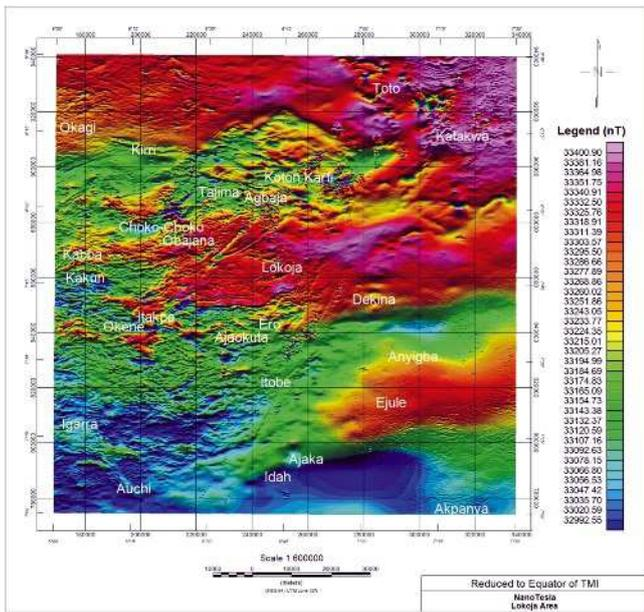
Fig. 2: Reduced to equator of total magnetic intensity (RTE-TMI) anomaly map of the area.
