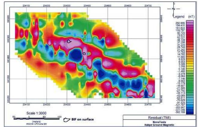
Fig. 5: Residual Magnetic intensity map of the Itakpe iron ore field.
