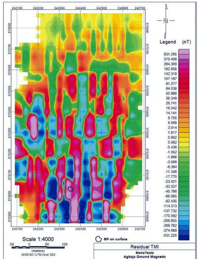
Fig. 7: Residual magnetic intensity map of the Agbaja iron ore field.
