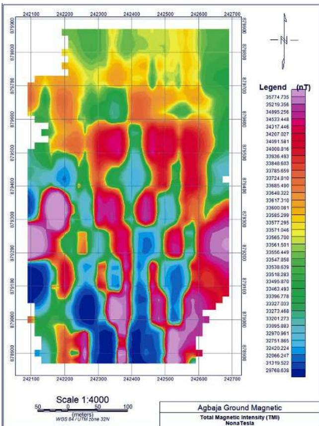
Fig. 6: Total magnetic intensity map of the Agbaja iron ore field.
