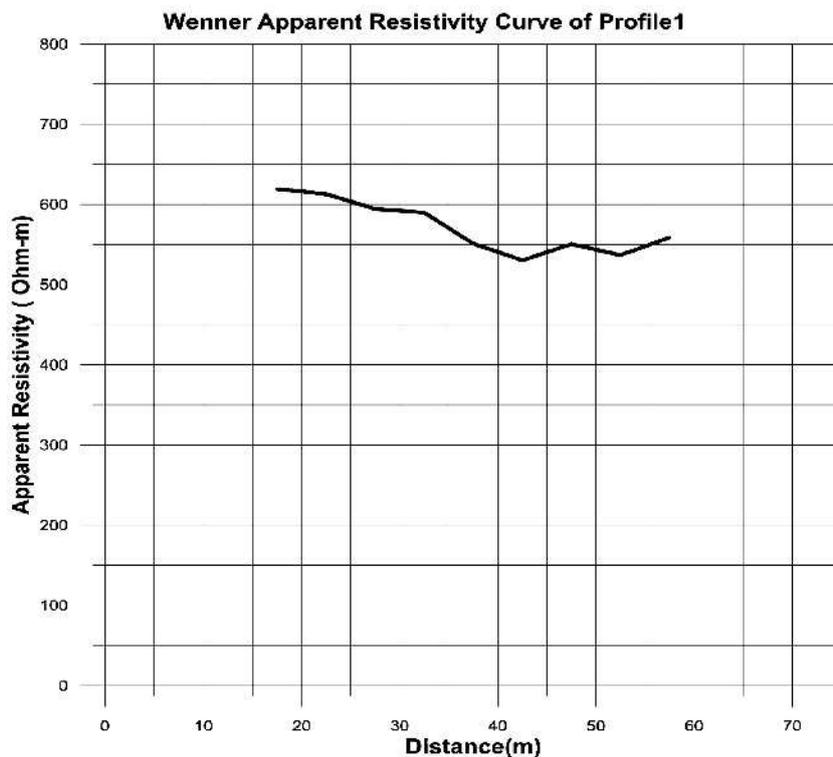
Fig. 8: Wenner apparent resistivity curve for profile1
