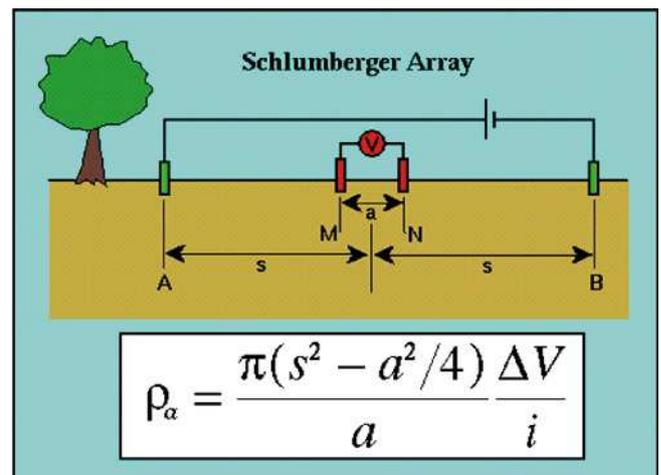
Fig. 4: The Schlumberger Array for an electrical resistivity survey
