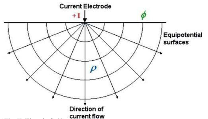
Fig. 5: Electric field at a point source
