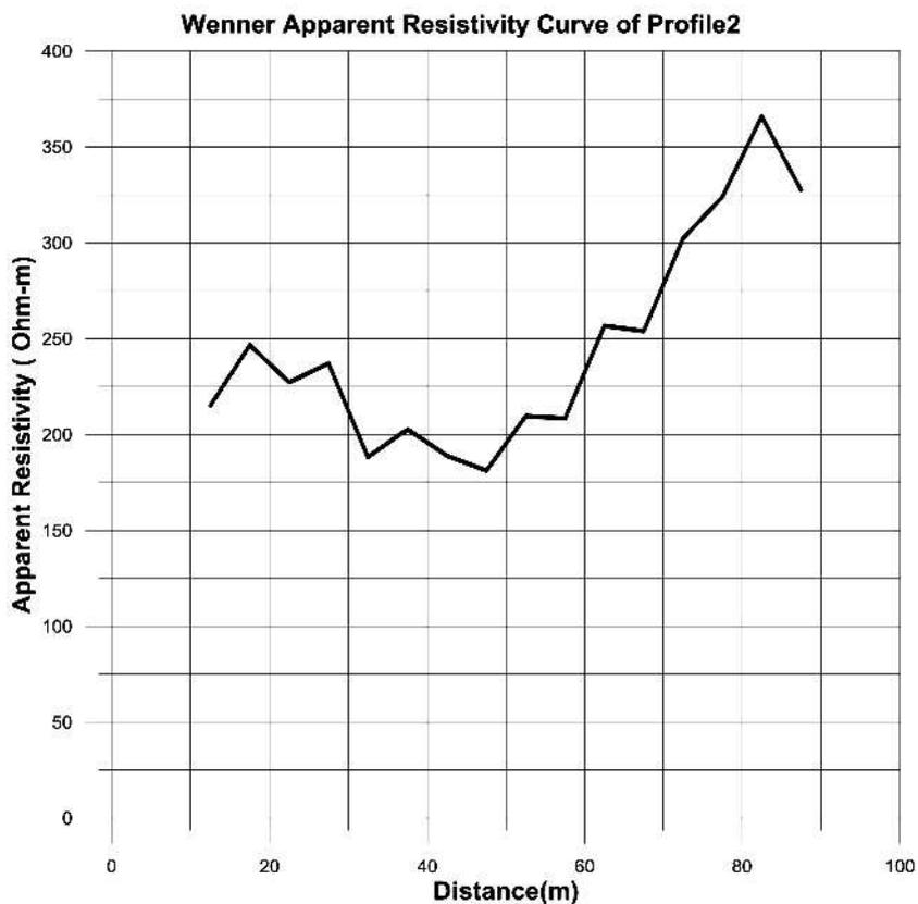
Fig. 9: Wenner apparent resistivity curve for profile 2
