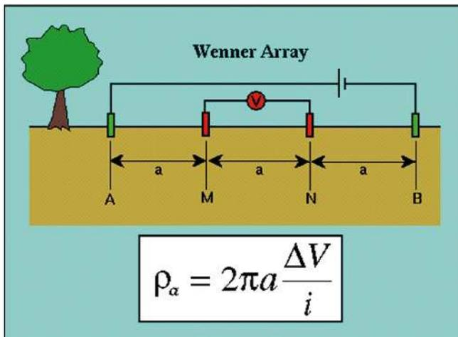
Fig. 3: The Wenner Array for an electrical resistivity survey.
