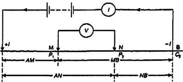
Fig. 6: General configuration of the four surface electrodes in linear resistivity surveys.
