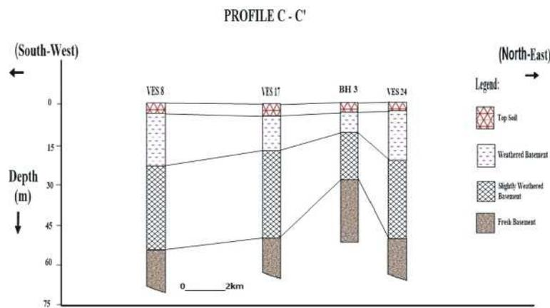
Fig. 17: Correlation of Borehole lithologic section (BH 3) and Geo - electrical sections (VES 8, VES 17 and VES 24) from profile C-C'.
