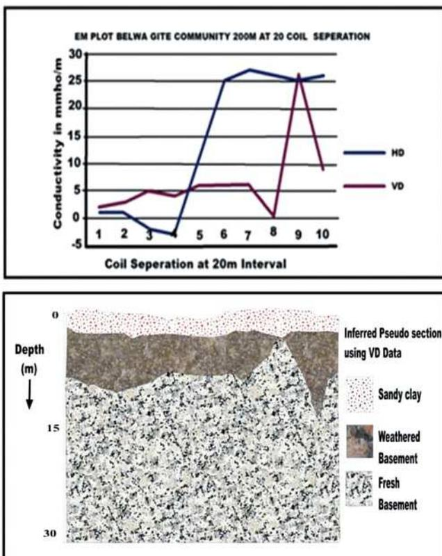
Fig. 6: EM/Geologic section of Belwa
