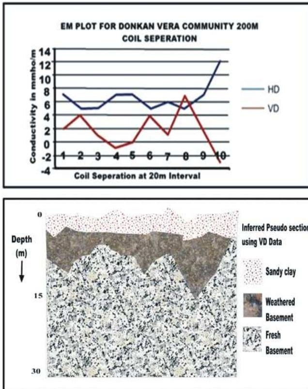
Fig. 5: EM/Geologic section of Donkan
