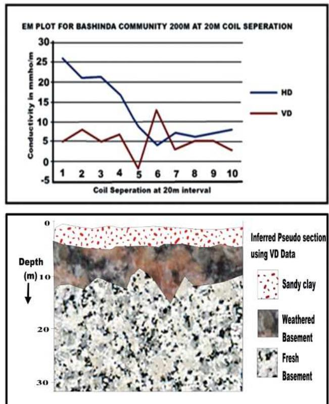
Fig. 8: EM/Geologic section of Bashinda
