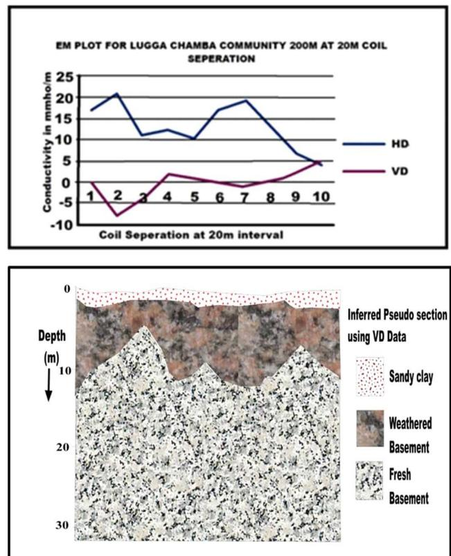
Fig. 7: EM/Geologic section of Lugga Chamba
