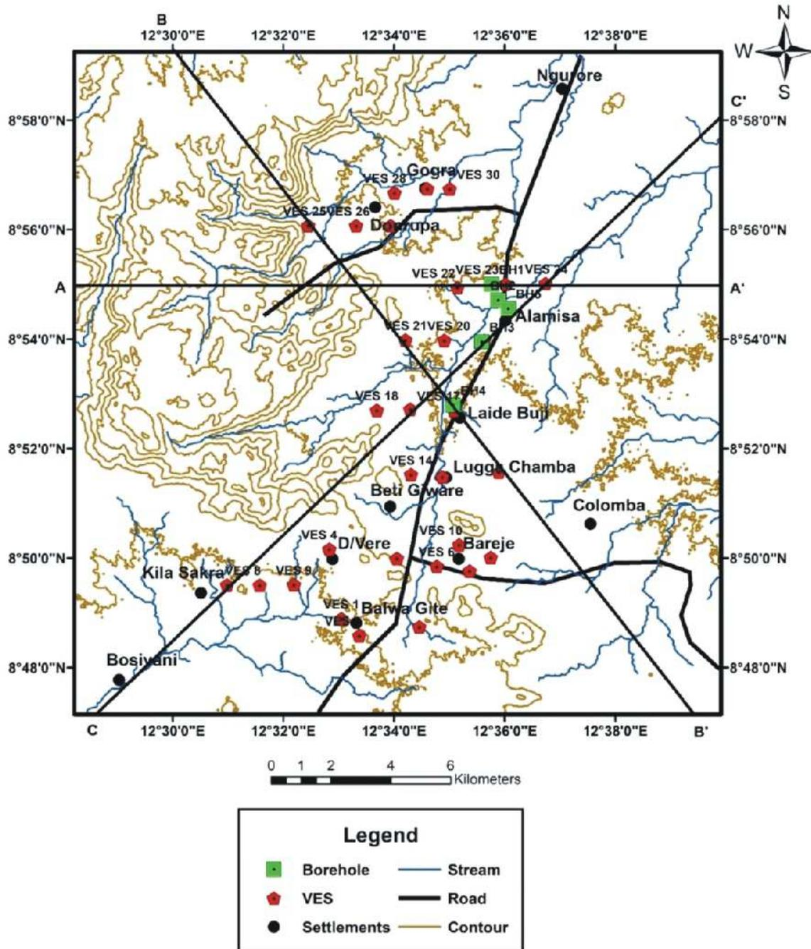
**Fig. 14:** Location of correlated lines along A-A', B-B' and C-C' with VES points and existing boreholes (1, 2, 3, 4 and 5)
