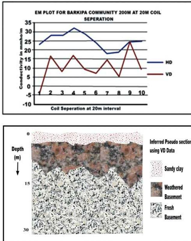
Fig. 10: EM/Geologic section of Alarba Gurigwa
