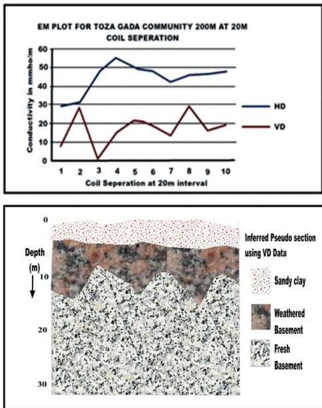
Fig. 9: EM/Geologic section of Toza Gada
