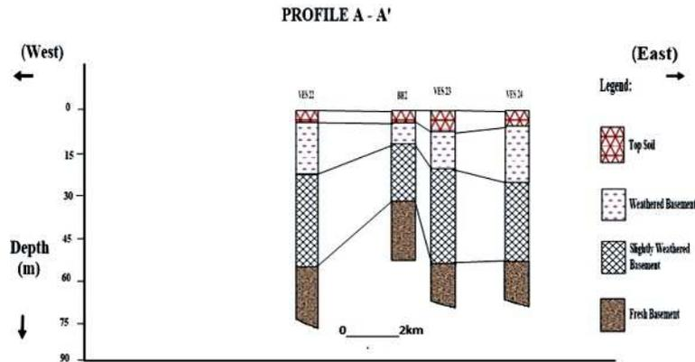
Fig. 15: Correlation of Borehole lithologic section (BH 2) and Geo - electrical sections (VES 22, VES 23 and VES 24)
