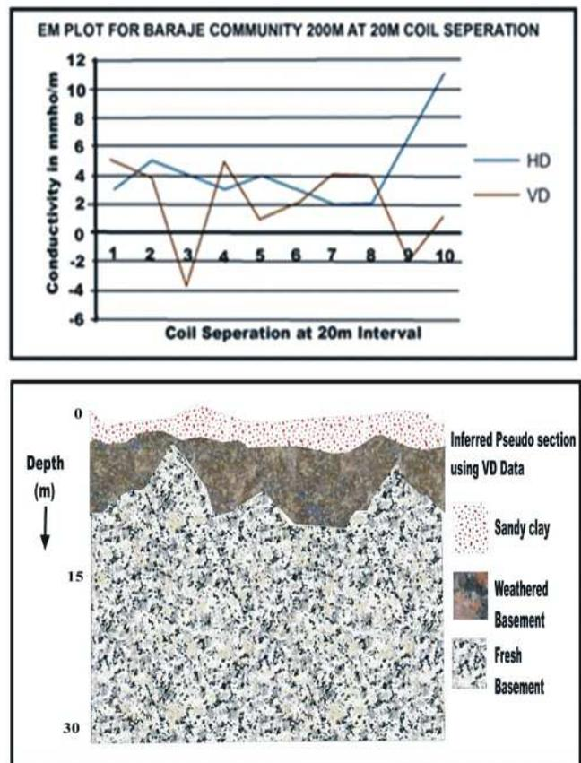
Fig. 4: EM/Geologic section of Baraje
