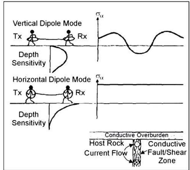
Fig. 3: Field arrangement for vertical and horizontal dipole position in electromagnetic (EM) survey (Geonics Limited 50<sup>th</sup> Anniversary, 1962-2012)
