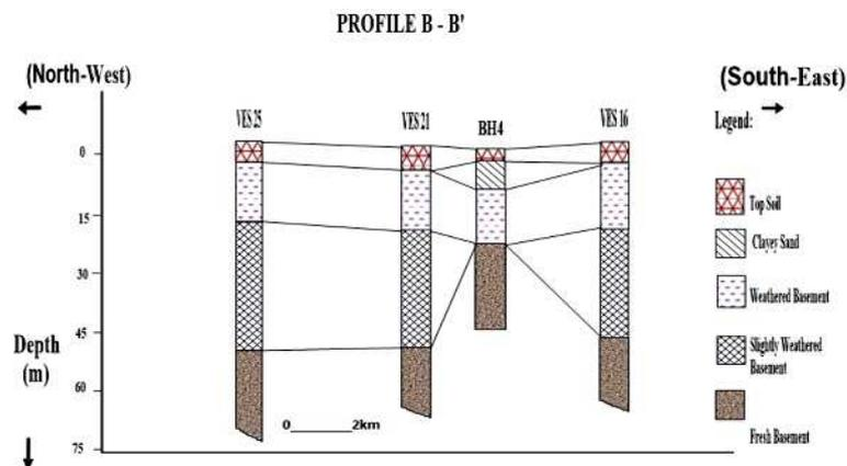
Fig. 16: Correlation of Borehole lithologic section (BH 4) and Geo - electrical sections (VES 16, VES 21 and VES 25)
