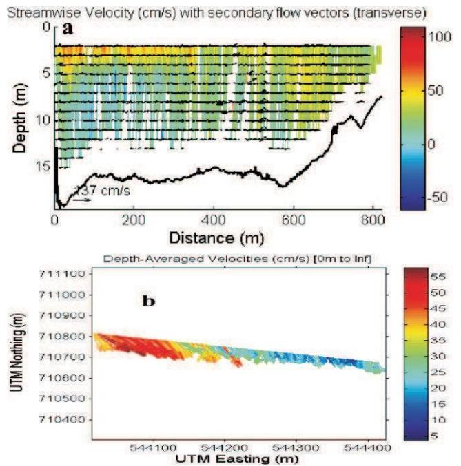
**Fig. 8:** (a) Streamwise velocity profile, (b) Depth average velocity profile
