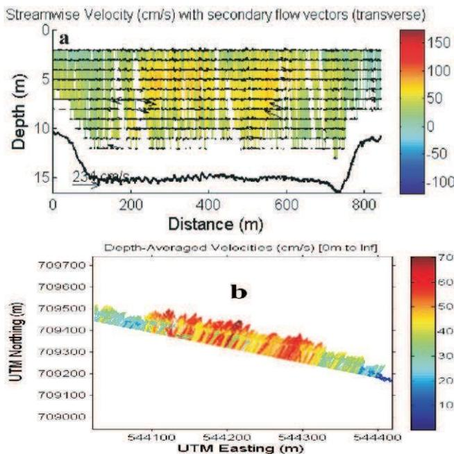
**Fig. 7:** (a) Streamwise velocity profile, (b) Depth average velocity profile
