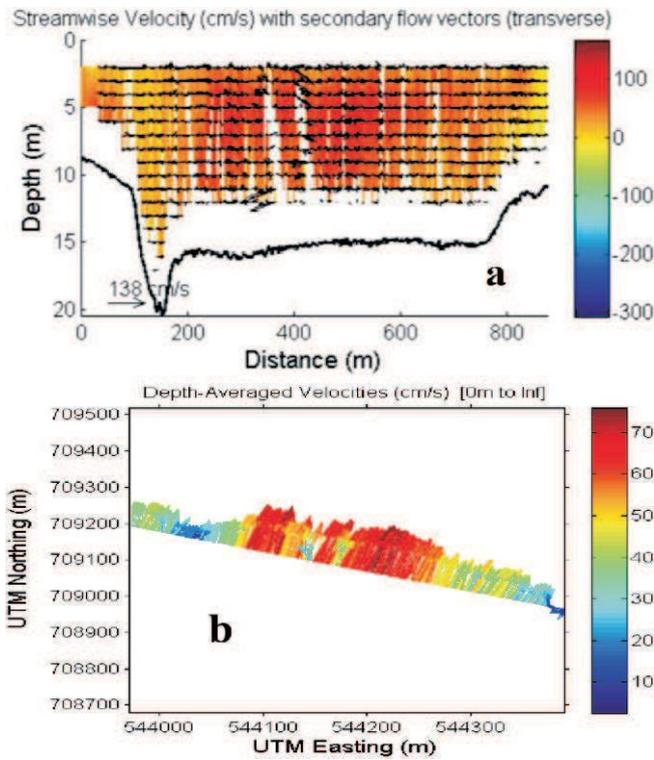
**Fig. 6a:** (a) Streamwise velocity profile, (b) Depth average velocity profile velocity magnitude of between 0.1 to 0.5 m/sec, over a depth ranged of 2 to 15 m. Maximum velocity was recorded within the channel centre while minimum velocity was recorded along the channel banks (Figure 7a). The depth average velocity DAV vectors was pointing north indicated a flood flow direction (Figure 7b).
