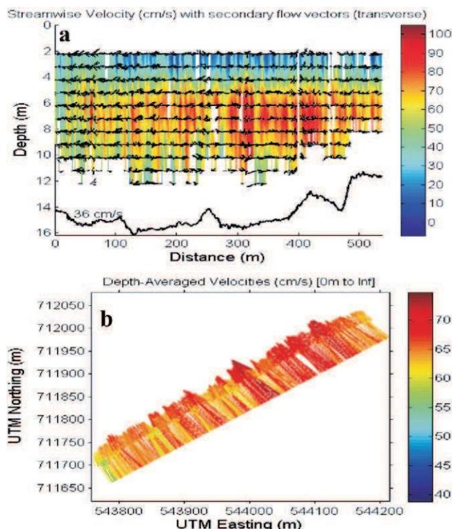
Fig. 9: (a) Streamwise velocity profile, (b) Depth average velocity profile
