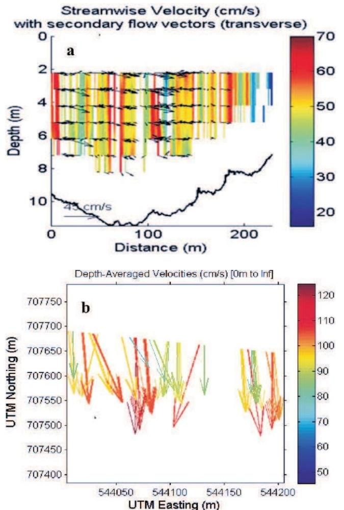
Fig. 5: (a) Streamwise velocity profile, (b) Depth average velocity profile
