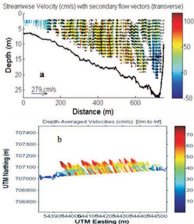
Fig. 4: (a) Streamwise velocity profile, (b) Depth average velocity profile
