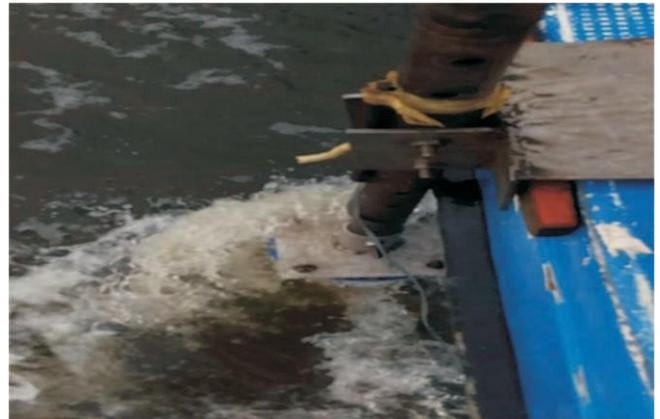
**Fig. 3a:** ADCP deployed in water
