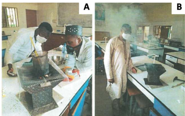
Fig. 7: Ogboyaga coal combustion showing stained beaker (A) and significant smoke emission(B)
