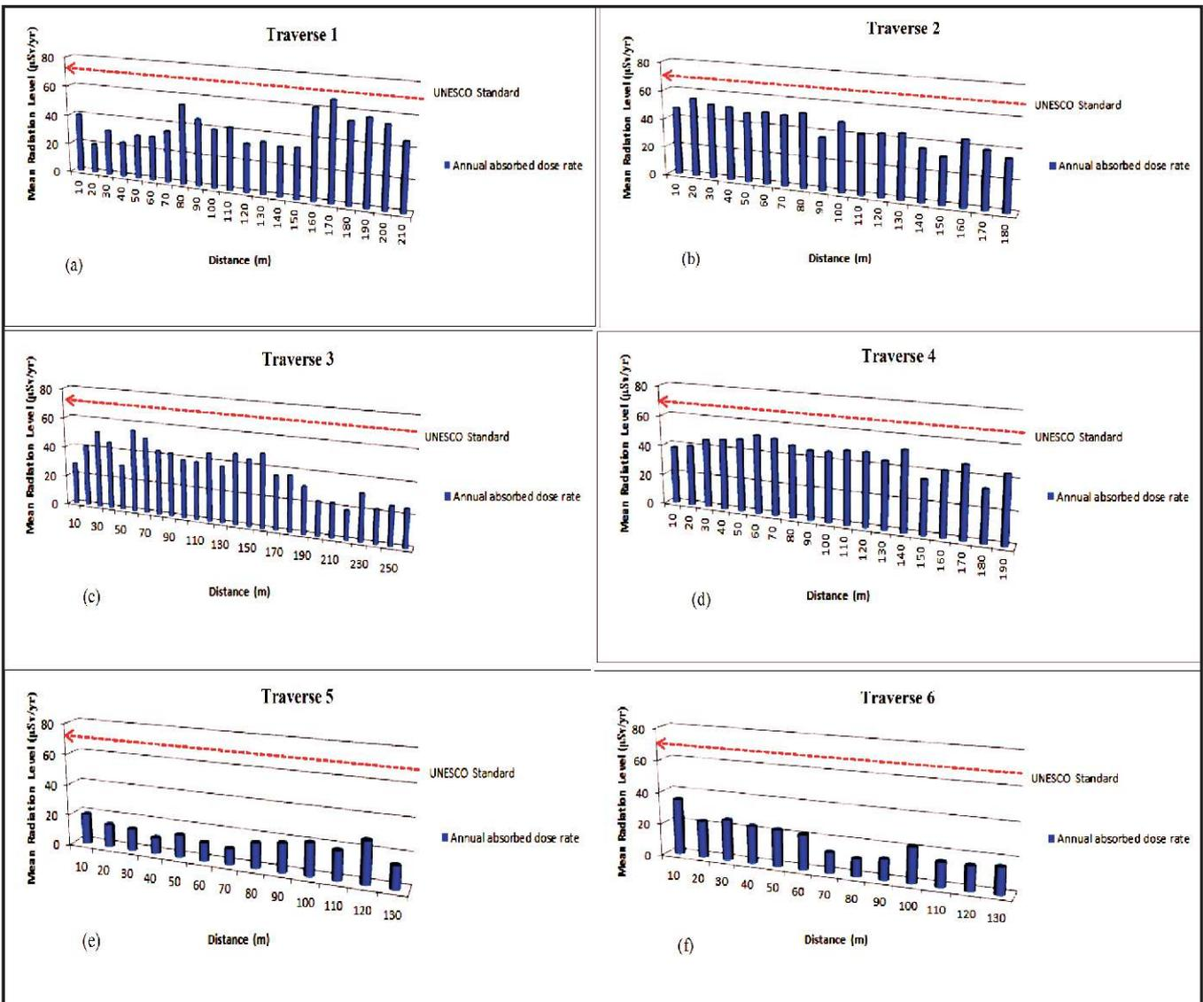
Fig. 14: Measured Radiation level versus Normal Background along Traverses 1-6.
